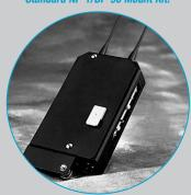
Allows ENG-100 to be mounted on a standard NP-1 or BP-90 battery holder. Can be easily installed and removed with thumb screws.
